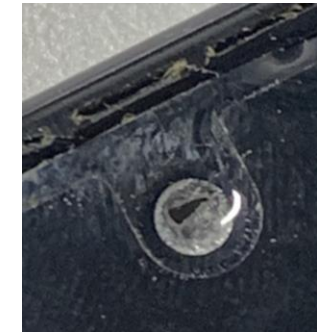
Punctured camera window
