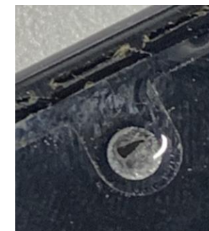
Punctured camera window
